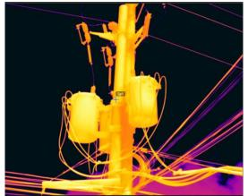
Thermography is a non-destructive test method that used to detect poor connections, unbalanced load, deteriorated insulation or other potential problems in energized electrical components including power transformer.
